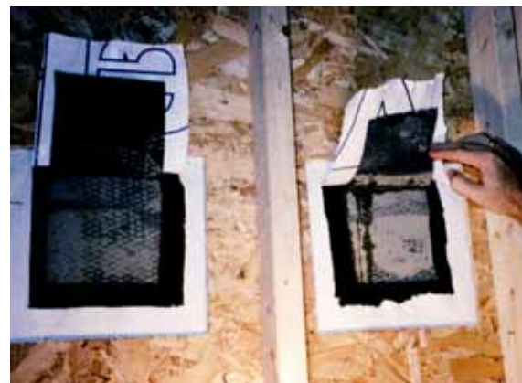
Photograph 7: Building Paper Bond Break —Traditional building paper is an excellent bond break between traditional hardcoat stucco and plastic building papers.
